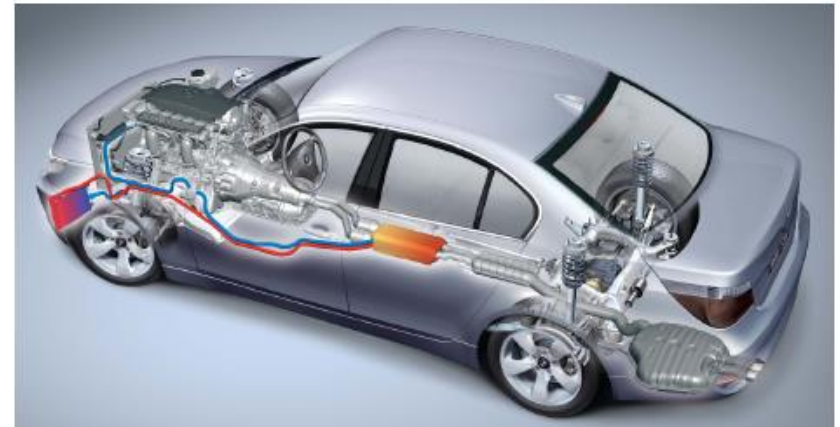
BMW Series 5, Model Year 2010, 3.0 Liter Gasoline Engine w/ Thermoelectric Generator
